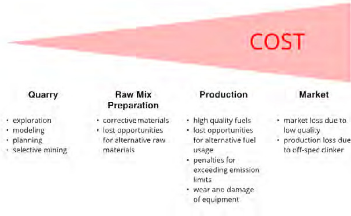
Figure 4 Cost for correction or mitigation of quality deviations at different stages of cement production between quarry and market
